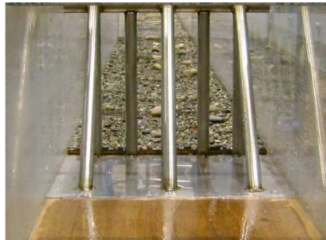
Gambar 6. Model cek dam terbuka di flume laboratorium
